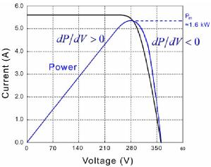
**Fig. 5.** Output characteristic curve of photovoltaic array strings.
