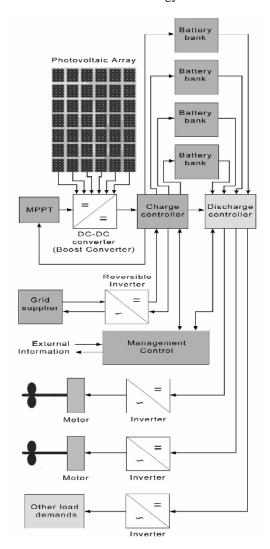
Fig. 4. Topology of solar-electric boat.
