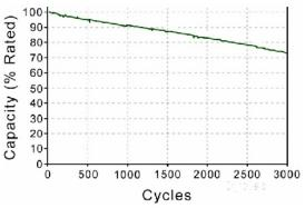
Fig. 3. Valence U27-36XP capacity retention.
